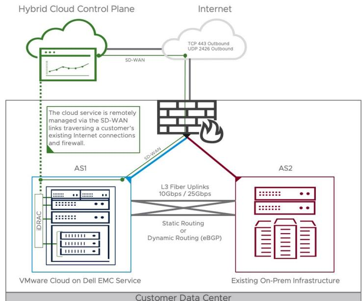
FIGURE 5. VMware Cloud on Dell EMC networking overview
